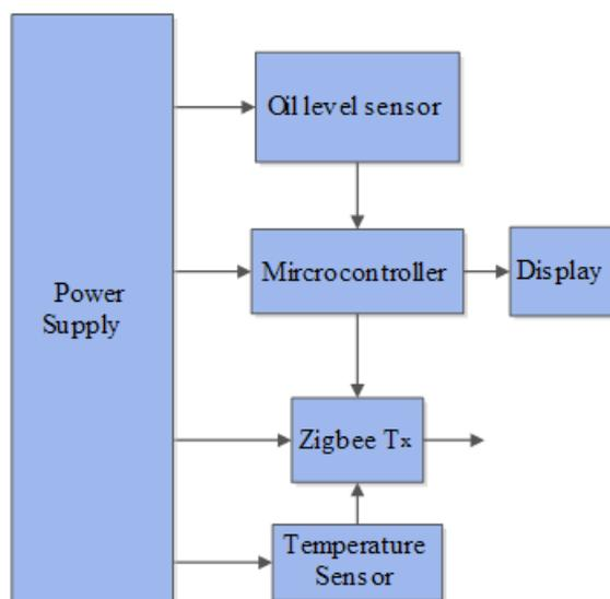
**Fig 1.** Block diagram of the end device
