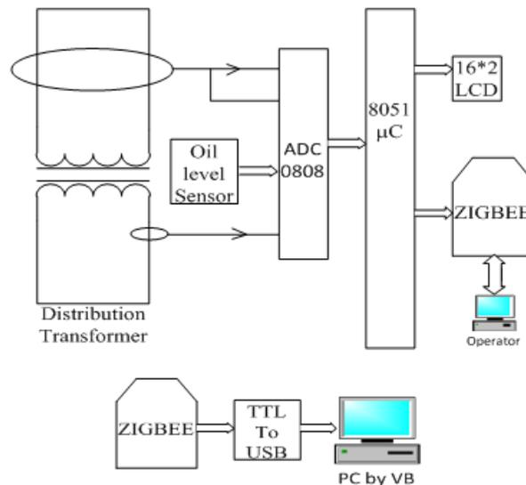
**Fig. 3.** The hardware structure for the ZIGBEE based transformer protection
