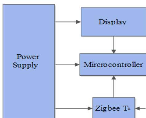
**Fig.2.** Block diagram of the coordinator unit
